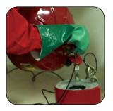
Safety cans transfer liquids through a bonding wire or earth lead for safe operation and control (bonding wire or earth lead is optional)
