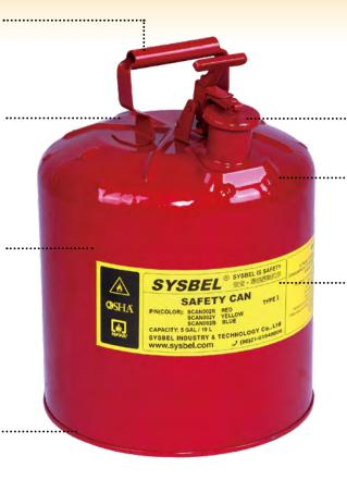
Positive press relief cap, leaktight, automatically vent vapor between 0.2 and 0.35bar(3 and 5 psig) to prevent rupture(or explosion in event of fire), spring loaded, it closes automatically after filling or pouring
